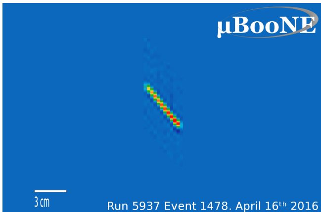
FIG. 9. Proton track candidate in MicroBooNE data. The track was selected by the decision tree classifier as being very likely a proton.
