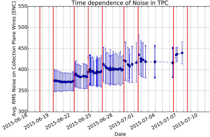
Figure 6: Noise on collection-plane wires at different times during the filling process. Vertical lines represent the approximate time of each fill. Data-points represent the mean noise value measured on collection-plane wires passing the cuts in Sec. 2. Error-bars show the standard-deviation of the noise on these channels and give a sense of channel-to-channel gain variations.
