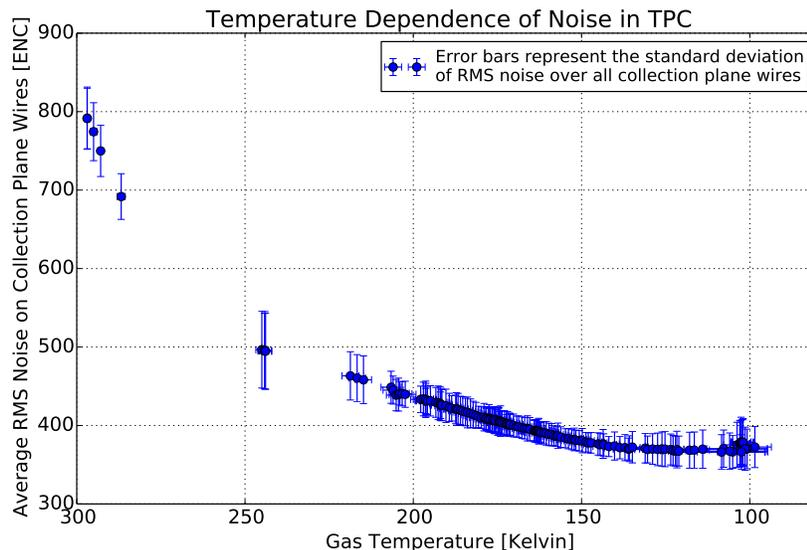
Figure 4: Noise on collection-plane wires vs. gaseous argon temperature inside the  $\mu$ BooNE cryostat. Noise measurements are shown in equivalent noise charge. Each data point shows the average RMS-noise value on collection-plane wires for each run. Error bars correspond to the spread in RMS-noise values due to channel-to-channel variations. Only channels passing the cuts described in Sec. 2 were used.
