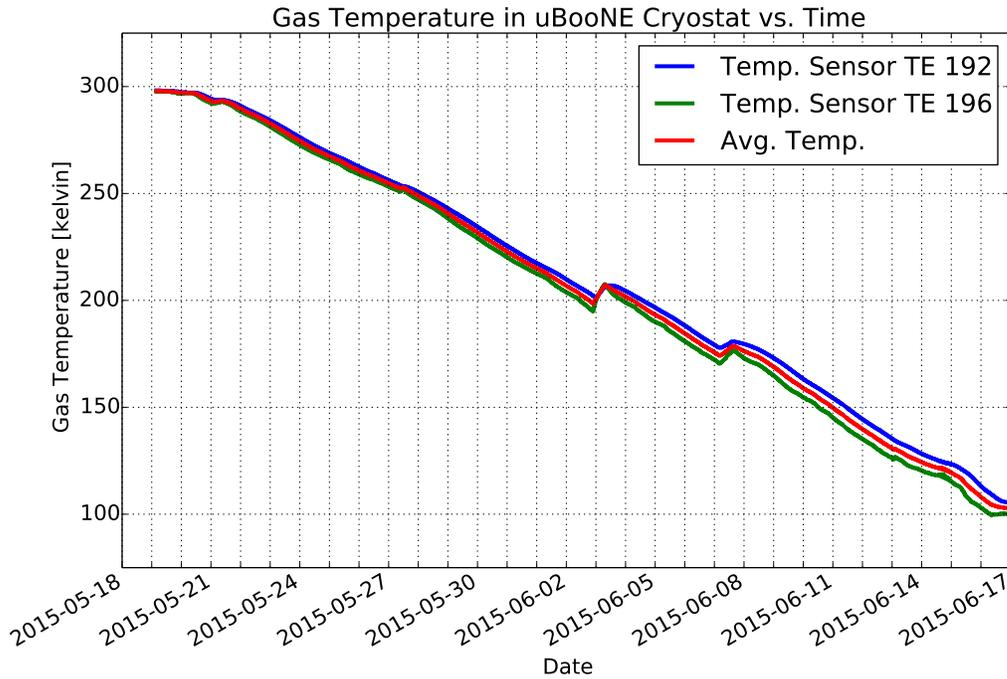
Figure 2: Temperature in the  $\mu$ BooNE cryostat over the course of the cool-down. Sensors TE192 and TE196 were located on the top and bottom of the TPC frame, respectively. In red we show the average of the two, used in this analysis.
