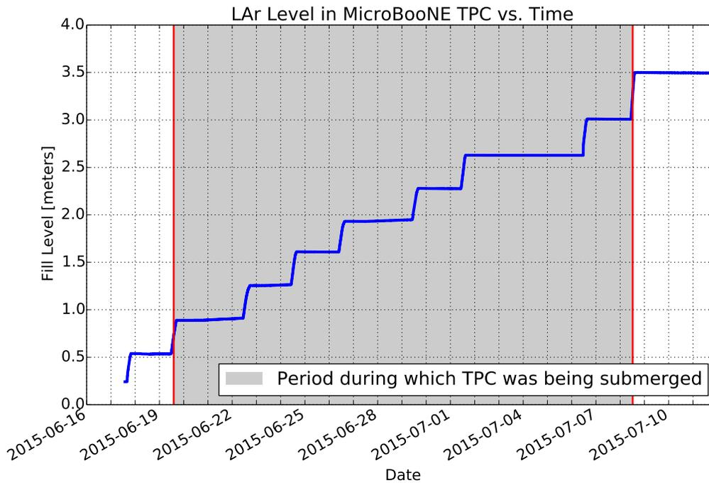
Figure 5: LAr fill level over the several weeks during which the filling process occurred. The fill level is measured relative to the bottom of the cryostat in meters. The fill level is calculated from a gas-pressure measurement in the TPC. The shaded grey area marks the time in which the LAr level fell between the bottom and top of the TPC frame. Each step in this plot marks the approximate time of a fill.
