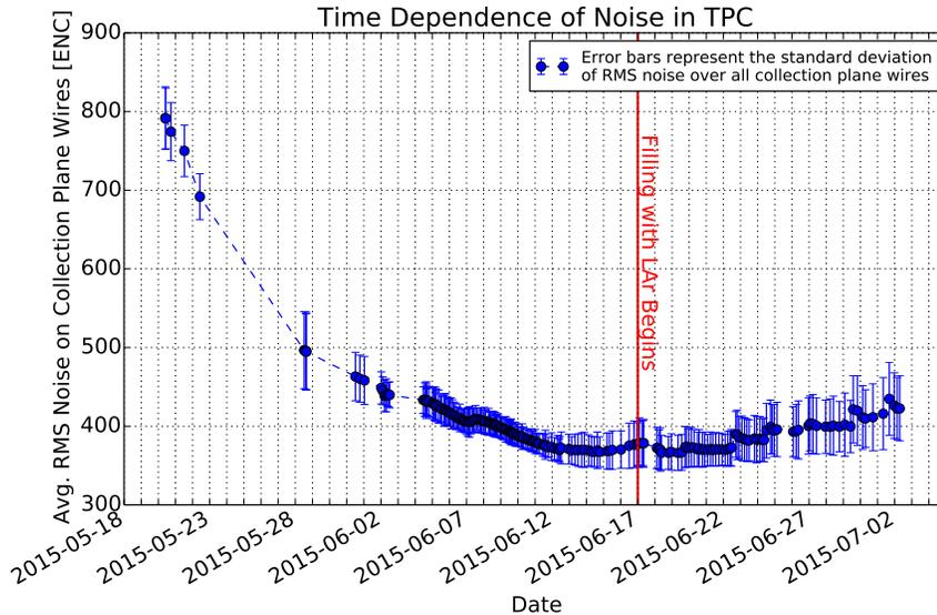
Figure 3: Noise measured on collection plane wires as a function of time. Each data point corresponds to the measured noise level for a given run. The times shown are the times of each run. Data points and error bars are the average and standard deviation, respectively, of the distribution of RMS values measured on collection-plane wires. The vertical red line marks the date on which the LAr filling began.
