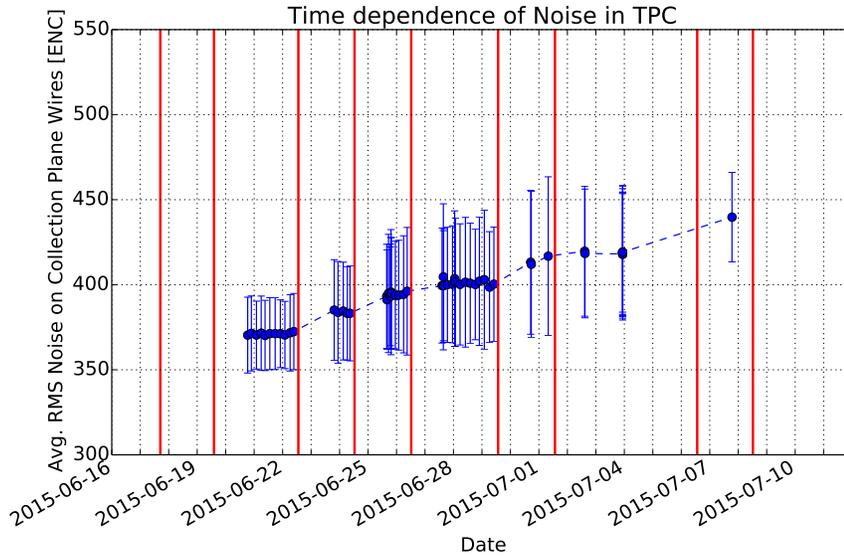
Figure 7: Noise on collection-plane wires at different times during the filling process. Vertical lines represent the approximate time of each fill. Runs taken 3 hours before or 24 hours after a fill were removed. Additionally, runs taken when the LAr level was below or above the top of the TPC were also removed.
