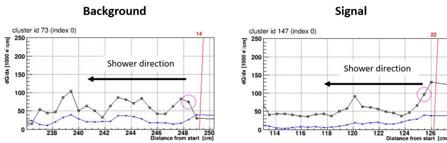
**Figure 19:** Illustration of MIP identification for EM showers. (Left) A background event. The MIP  $dQ/dx$  is expected to be around 45k electrons/cm. (Right) A signal event with a high  $dQ/dx$  at the neutrino interaction vertex. The blue lines give a measure of the fit quality. The red line with a number is used to separate the different track segments. The identified neutrino vertices happen to be at larger distance from the start for these two examples.
