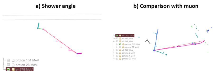
**Figure 22:** (Left) An EM shower going backward with respect to the neutrino beam direction. (Right) A long muon is found in addition to the electron candidate. The grey box represents the MicroBooNE active TPC volume, which is 2.56 m in the drift direction (X), 2.3 m high (Y), and 10.56 m along the beam axis (Z).
