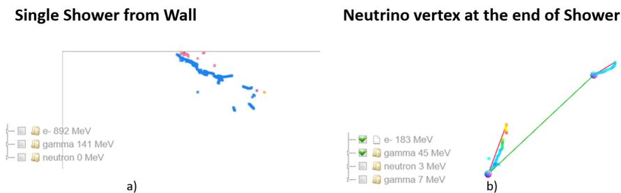
**Figure 20:** Illustration of single EM showers. (Left) An EM shower close to the top of the detector. (Right) The neutrino vertex is misidentified to be at the end of EM shower. The grey box represents the MicroBooNE active TPC volume, which is 2.56 m in the drift direction (X), 2.3 m high (Y), and 10.56 m along the beam axis (Z).
