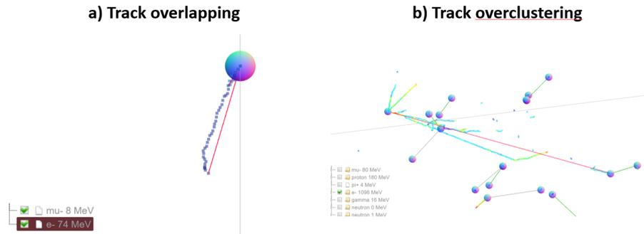
**Figure 24:** (Left) An overlapping situation at the beginning of EM shower's stem region. (Right) An example of track overclustering situation. One of the tracks clearly shows the Bragg's peak. The grey box represents the MicroBooNE active TPC volume, which is 2.56 m in the drift direction (X), 2.3 m high (Y), and 10.56 m along the beam axis (Z).
