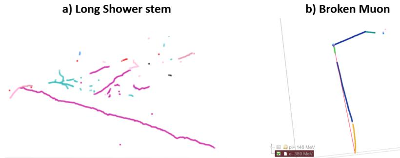
**Figure 21:** (Left) The identified EM shower has a long stem, which indicates an over-clustering situation (e.g. with a muon). (Right) A long muon is broken into pieces, which leads to a misidentification. The grey box represents the MicroBooNE active TPC volume, which is 2.56 m in the drift direction (X), 2.3 m high (Y), and 10.56 m along the beam axis (Z).
