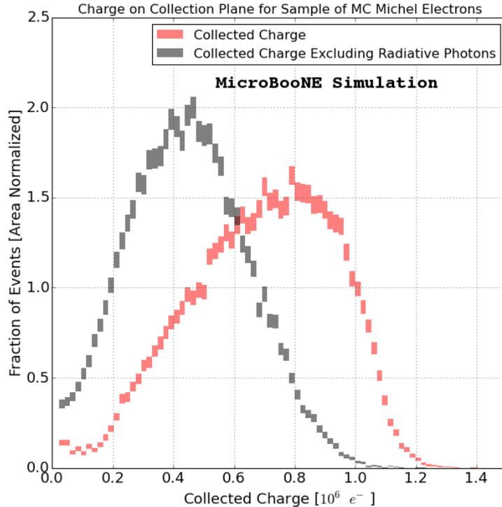
Figure 6: Distribution of charge collected on the TPC collection plane for a sample of Monte Carlo Michel electrons. The two curves show the collected charge when including (red) and excluding (black) the charge that is deposited by the byproducts of radiative photons. The slight rise at very low deposited charge in the distributions is due to Michel electrons that escape the TPC at least in part, and for which only a fraction of their deposited energy drifts to the collection plane.
