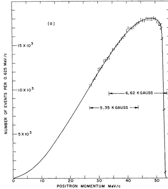
Figure 2: Reconstructed Momentum spectrum of positrons from decay-at-rest muons produced by a positive pion beam from the Columbia University cyclotron at the Nevis laboratories [3].
