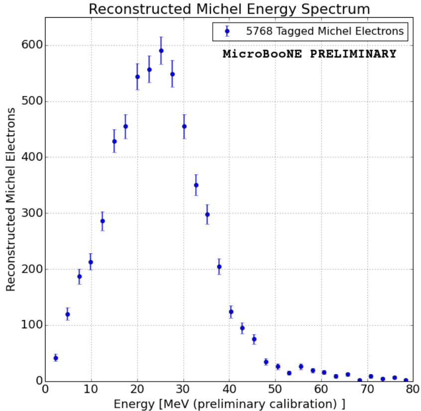
Figure 11: Reconstructed Michel electron Energy Spectrum produced using cosmic data taken with the MicroBooNE detector. Error bars represent statistical uncertainties only.
