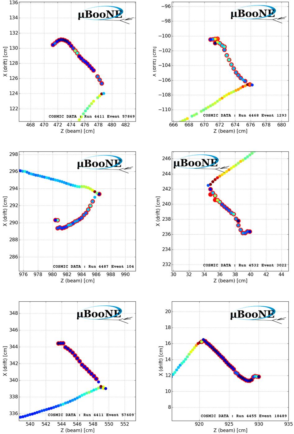
Figure 9: Event displays of tagged Michel electrons from data. Each image shows the reconstructed hits in the wire,time view of the collection plane in the vicinity of a tagged Michel electron. Hit charge (measured in ADC x Tick) is represented by the hit color. Charge increases as the color moves from blue to red. Hits tagged as belonging to a Michel electron are outlined in red.
