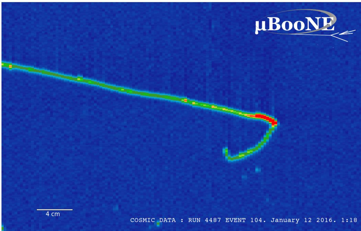
Figure 3: Event display showing raw data for a region of the collection plane associated with a candidate Michel electron. Wire-number is represented on the horizontal axis, and time on the vertical. Color is associated with the ADC count on each channel.
