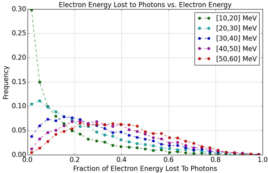
Figure 5: Fraction of an electron’s energy lost to radiative processes. For each energy range a large number of electrons was simulated in the detector. For each electron, the fraction of energy transferred to “primary” photons (photons to which energy is transferred directly by the original electron) is calculated. Each curve shows the distribution of such energy transfers for electrons in a given energy range.
