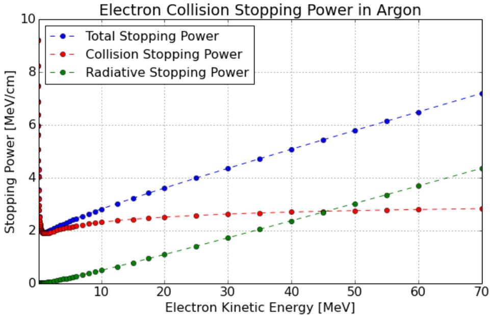
Figure 4: National Institutes of Standard and Technology (NIST) stopping power data for argon [4]. Collision stopping power denotes energy lost by electron ionization. Radiative stopping power indicates the average energy lost to photons via electron Bremsstrahlung.
