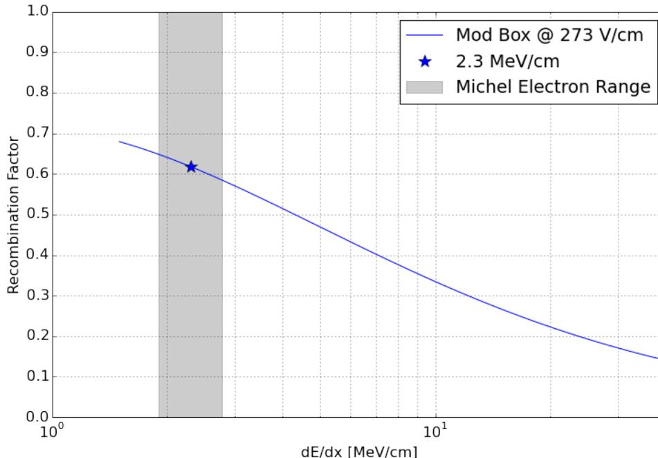
Figure 10: Recombination factor as a function of  $dE/dx$  calculated using the Modified Box model as described by ArgoNeuT [5].
