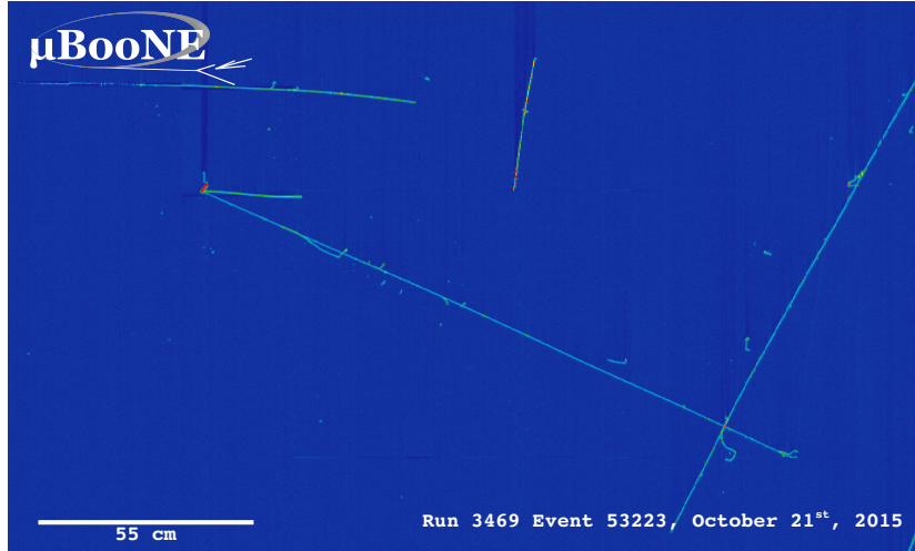
Figure 3: Neutrino interaction candidate event from MicroBooNE. Run 3469, event 53223, collection plane view. This event passed the optical + 3D-based TPC selection.
