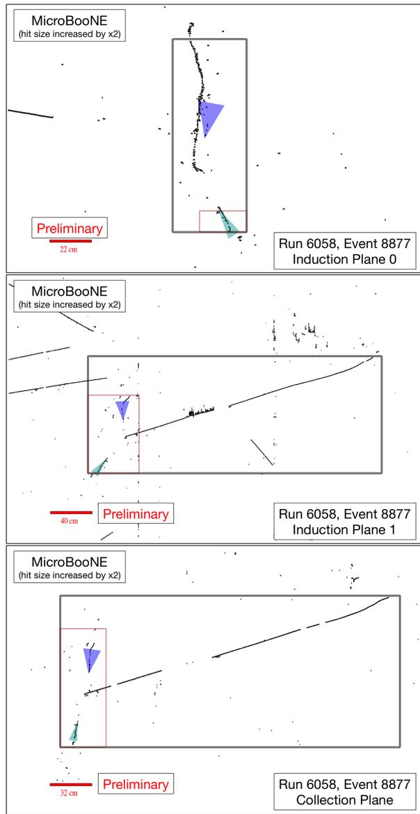
**FIG. 9:** Run 6058, Subrun 177, Event 8877, The green and blue triangles show the reconstructed showers associated with the  $\pi^0$  decays. Both appear to have been well reconstructed. The red box overlaid is the ROI which helps to guide the shower reclustering.
