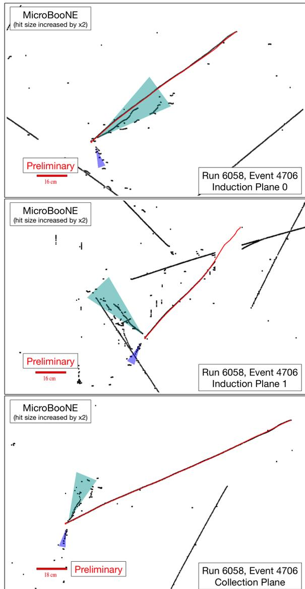
**FIG. 5:** Run 6058, Subrun 94, Event 4706, The green and blue triangles show the reconstructed showers associated with the  $\pi^0$  decays. Both appear to have been well reconstructed. The red track corresponds to the muon selected by the  $\nu_\mu$  filter.
