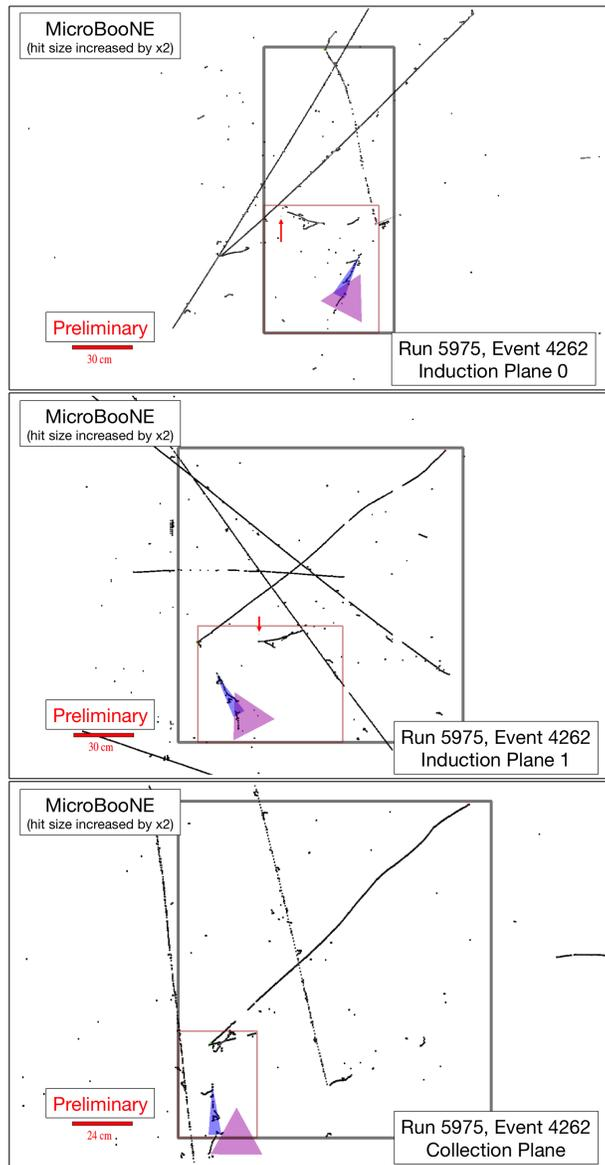
**FIG. 8:** Run 5975, Subrun 85, Event 4262, Three showers are reconstructed in this event: a blue and red one, associated with the same EM shower, which was broken up in the reconstruction. A third, very small green shower associated with the green cluster (highlighted by the red arrow) can be found. The red box overlaid is the ROI which helps to guide the shower reclustering.
