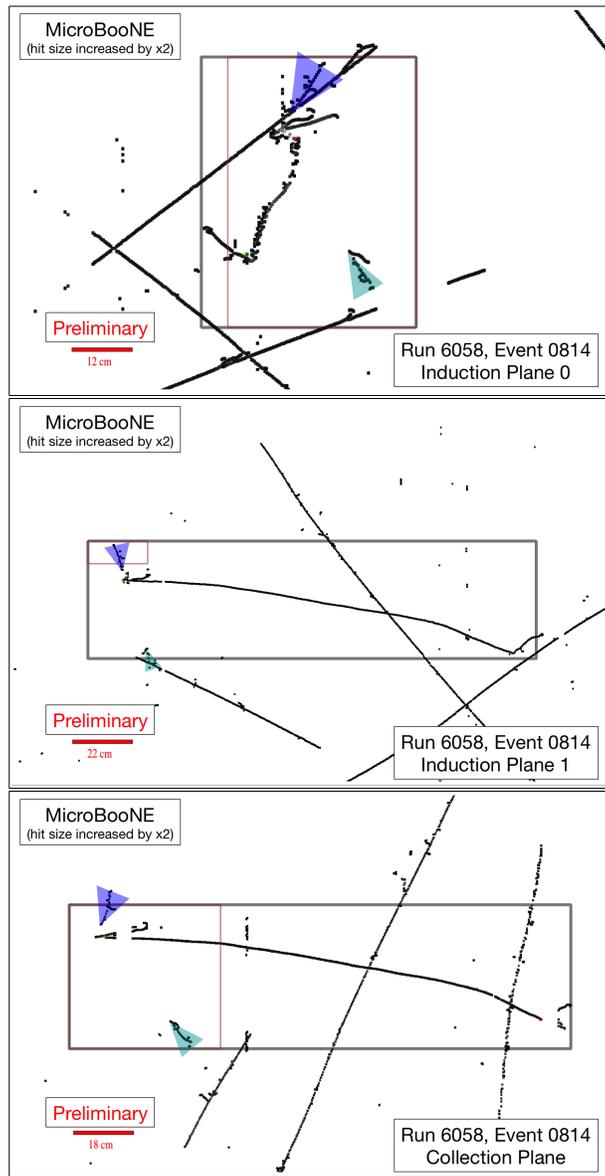
**FIG. 11:** Run 6145, Subrun 16, Event 814, The green and blue triangles show the reconstructed showers associated with the  $\pi^0$  decays. Both appear to have been well reconstructed. The red box overlaid is the ROI which helps to guide the shower reclustering.
