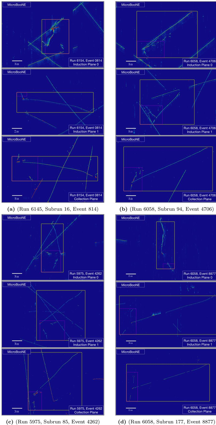
**FIG. 2:** Four MicroBooNE events selected from data to test our shower reconstruction. These events are intended to contain a neutrino induced muon and two photon showers originating from the neutrino interaction vertex. The yellow box is the interaction-wide ROI while the red box is the shower-wide ROI, which attempts to encompass all the charge associated with the two shower-like objects.
