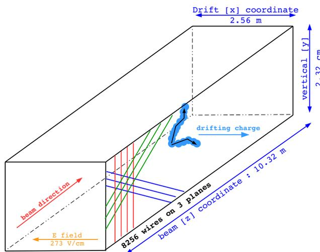
FIG. 1: A schematic of the MicroBooNE detector showing the coordinate system and wire planes.
