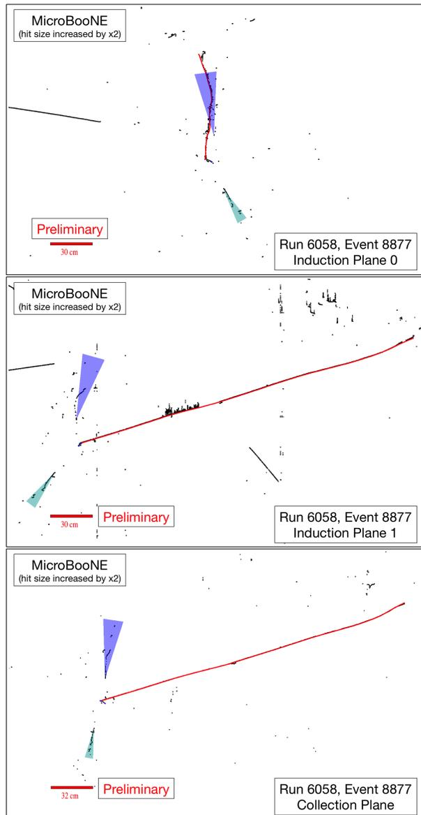
**FIG. 4:** Run 6058, Subrun 177, Event 8877, The green and blue triangles show the reconstructed showers associated with the  $\pi^0$  decays. Both appear to have been well reconstructed. The red track corresponds to the muon selected by the  $\nu_\mu$  filter.
