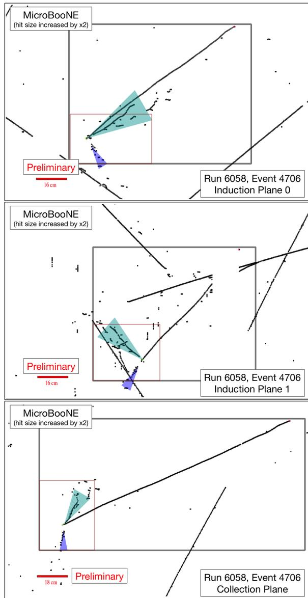
**FIG. 10:** Run 6058, Subrun 94, Event 4706, The green and blue triangles show the reconstructed showers associated with the  $\pi^0$  decays. Both appear to have been well reconstructed. The red box overlaid is the ROI which helps to guide the shower reclustering.
