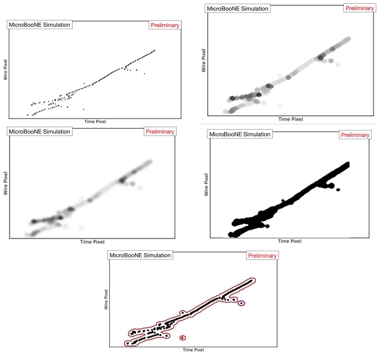
**FIG. 7:** From top left to right Original hits that make up a single cluster; Dilate pixels to “connect” nearby hits; Blur image to smooth edges and smear charge. From bottom left to right. Threshold converts grayscale image to binary; OpenCV contour finding on threshold image produces a polygon which now encloses the original hits.
