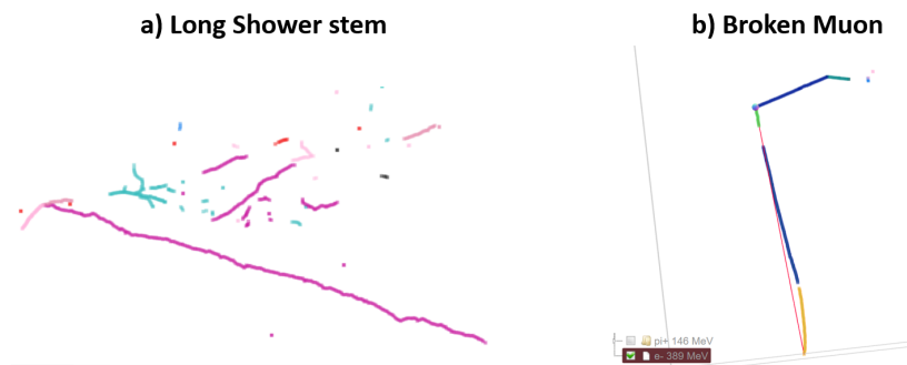
Figure 22: (Left) The identified EM shower has a long stem, which indicates an over-clustering situation (e.g. with a muon). (Right) A long muon is broken into pieces, which leads to a misidentification. The grey box represents the MicroBooNE active TPC volume, which is 2.56 m in the drift direction (X), 2.3 m high (Y), and 10.56 m along the beam axis (Z).
